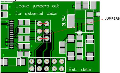
By removing the three jumpers external I2S data can be used. The data input has the following connections:
